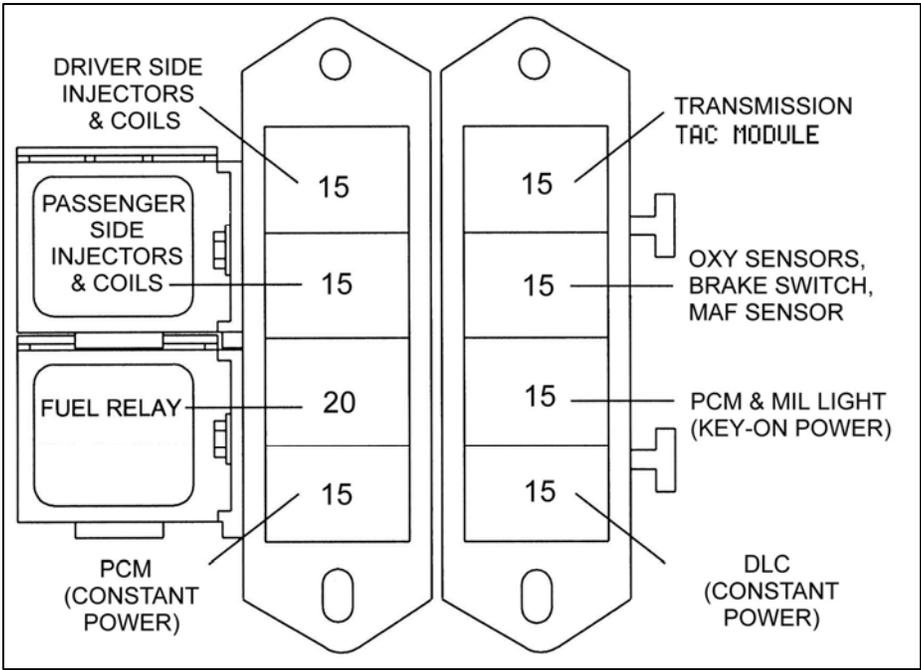
**FIGURE 7.1** 60522-23 Fuse Identification
