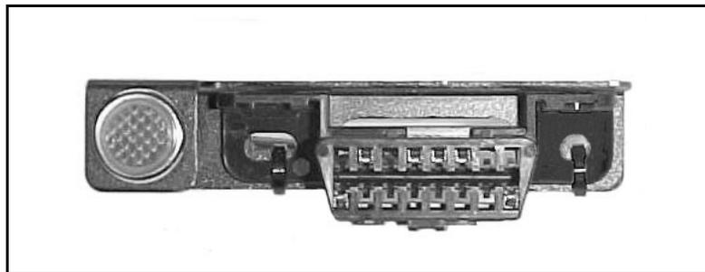
**FIGURE 6.1** DLC Connector & Check Engine Light
