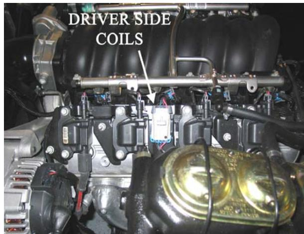
**FIGURE 6.18** Driver Side Coil Connector
