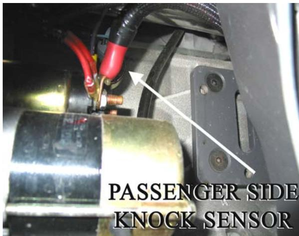
**FIGURE 6.23** Passenger Side Knock Sensor
