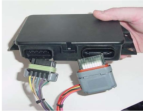
**FIGURE 6.22** TAC Module Connections
