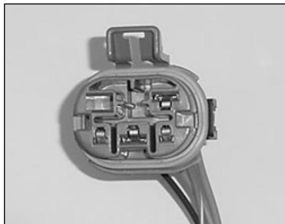
**FIGURE 6.5** Fuel Pump Relay Connector
