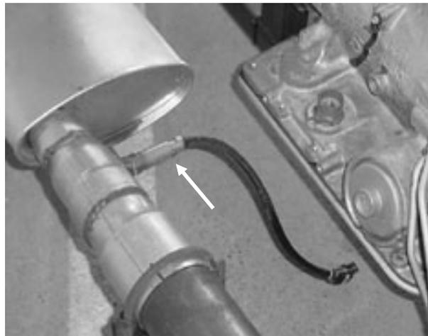
**FIGURE 6.9** Oxygen Sensors
